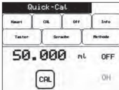
Customer calibration enables the user to calibrate his unit himself to exactly suit a special application case. 10 ml, 20 ml or 50 ml (depending on the unit) of the medium is dispensed for this purpose and then weighed on an adequately-accurate scale, with actual volume being calculated taking the density into consideration. The actual volume can now be entered in the
